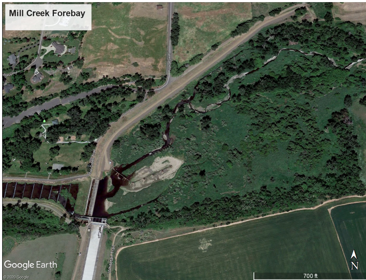
Figure 21 – Plan view of the Mill Creek diversion dam.
